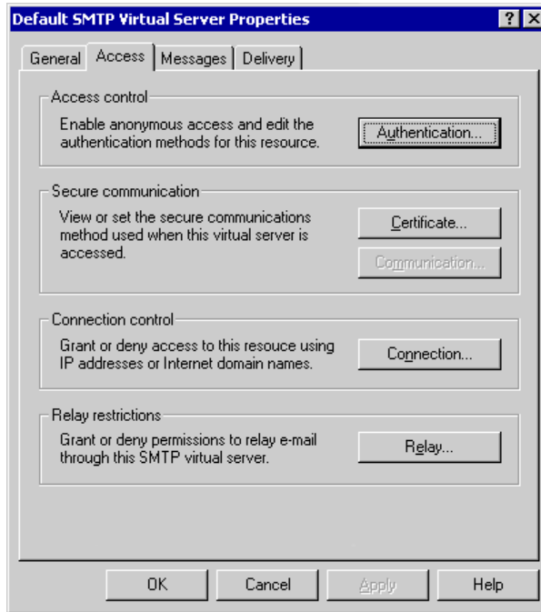
Figure 14 The Access tab in the Default SMTP Virtual Server Properties dialog box
